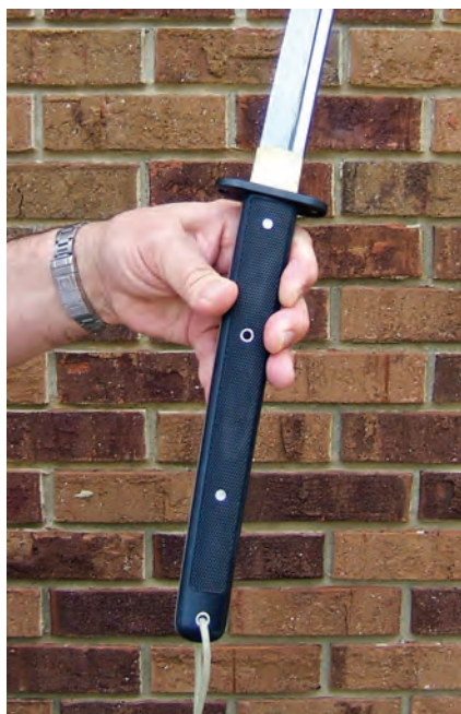
The handle slabs are anchored to the tang in four places.
