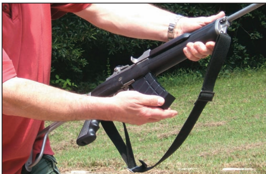
If you are new to the Mini-14—or, for that matter, the AK-47—always remember to start the magazine into the receiver by what amounts to hooking it at the front and rotating the magazine rearward and upward.
