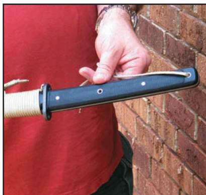
There are lanyard holes on the handle and on the guard, as well. The guard is small, but adequate to keep the hand from slipping forward onto the blade.
