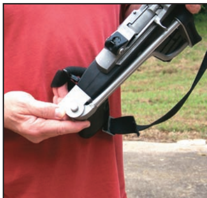
This button controls the locking and unlocking of the buttstock, whether folded or unfolded.
